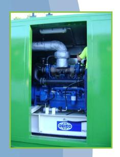
"Genpower Australia designed and manufactured the two co-joined container sets with access facility between the two containers and lift off doors. Each side had to meet OH&S standards for access of 900mm and weight of each door less than 25kgs each. These sets were built to specific site noise requirement of 65 dBA @ 7M as well as client colour.
